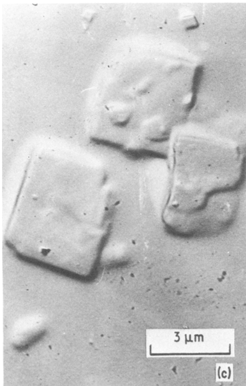
Figure 3 Transmission electron micrographs of thoria powder samples heated for 5 minutes at (a) 705, (b) 780 and (c) 825° C. The black blocks correspond to the crystallites extracted into the replica.
